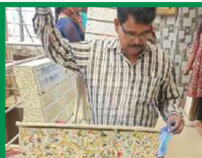
Benches being made of multi-layer plastic and tetra packs by Joshimath Nagar Palika Parishad
